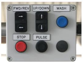
To raise gate: push up button, gate will rise to up position if no stop is pushed.
